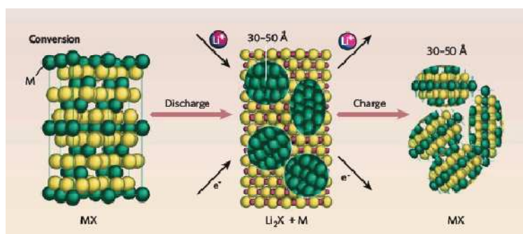
Figure 1: Schematic of the conversion reaction during discharge and charge of a lithium ion battery 4 .
